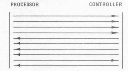
Eight peripheral controllers can be connected to the input/output bus. Each controller handles 8 peripherals which may be input or output or input/output devices.
